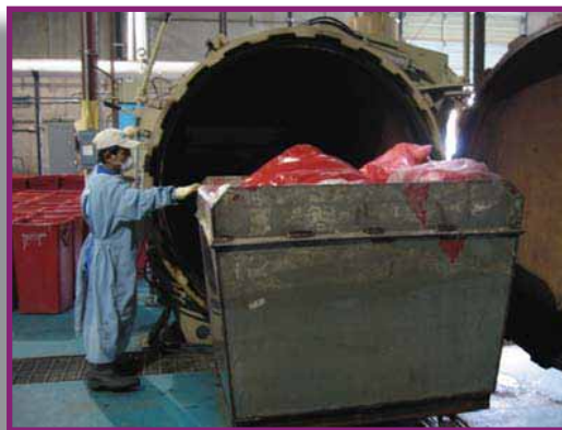
This autoclave will process five of these carts filled with biohazardous waste at one time.
